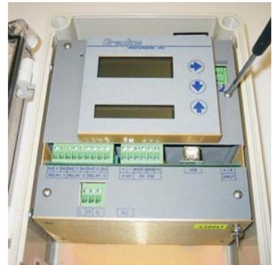
2. Remove the communications circuit board by gripping the USB connector and pulling upwards gently.
