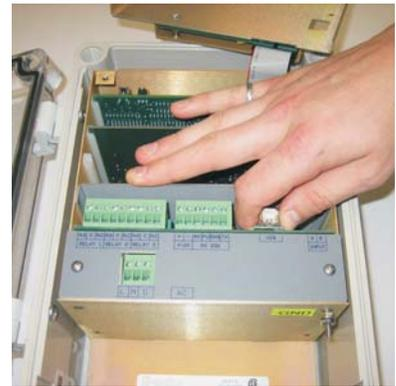
3. Locate the USB/RS232 links (Blue) on circuit board. Links are in the USB position by default. Move both links to the RS232 position for RS232 output.
